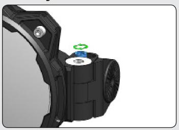
Loosen the M6 Socket-cap Adjustment Screws from End Mounts on both sides of the bar to allow alignment and self-centering.
