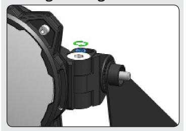
Set the final level and pitch of the Pro6: 1) Tighten the M8 Horizontal Mounting Hardware, allowing the Pro6 to center itself. Then, 2) Tighten the M6 End Mount Adjustment Screws to lock light into position.
