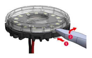
2. Insert flat head screwdriver and with slight pressure twist the screwdriver.
