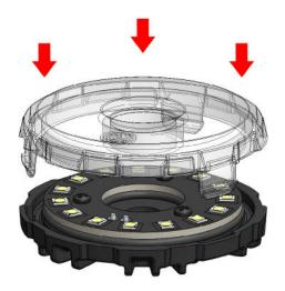
Press down firmly with equal pressure around the light to snap in new lens. (There should be no gaps between lens and light).
